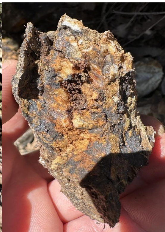
Figure 8 – Silver mineralisation within ferruginous quartz yielding 15.10 g/t Au from sample 3001037
