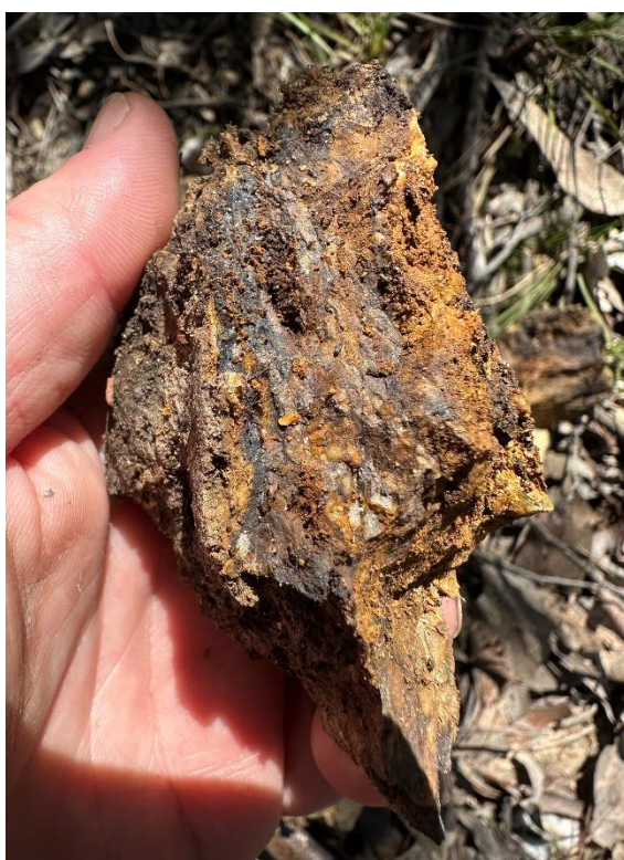
Figure 7 – Gold mineralisation within ferruginous rusty quartz yielding 24 g/t Au & 1.2 g/t Ag from sample 3001038
