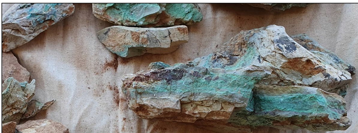
Photo 1. Rock chip sample KB03113, which returned 15.3% Copper 1 , comprised of oxidized white meta-tuffaceous siltstone with oxide copper mineralisation (green/dark grey in photo).
