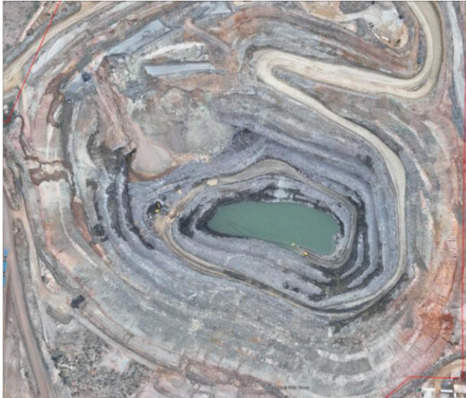
Greenfield Pit commissioned in May 2025 as in pit TSF with 4.5yr capacity @1.5Mtpa production rate
