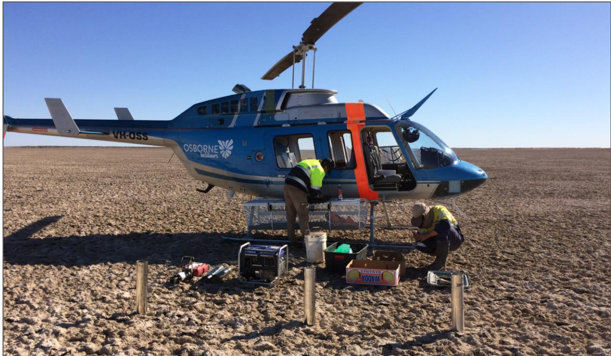
Figure 5. Shelby Tube Sampling in Progress
