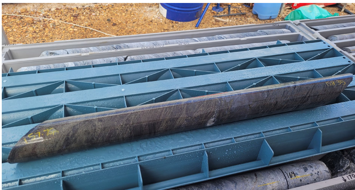
Figure 2: Photo of diamond drill core from GLPDD007 showing massive sulphide mineralisation grading into semi-massive sulphides with pyrite (yellow) and sphalerite (red) with galena and chalcopyrite. Associated sample interval GRD11022 (157.6-158.15m) returned 13.69g/t AuEq
