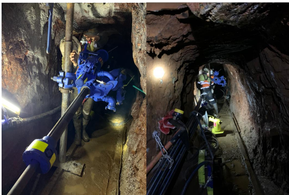
Figure 1: Kempe Drill set-up for drilling in Tyrconnel Access Adit, Blackwood Gold Exploration Project
