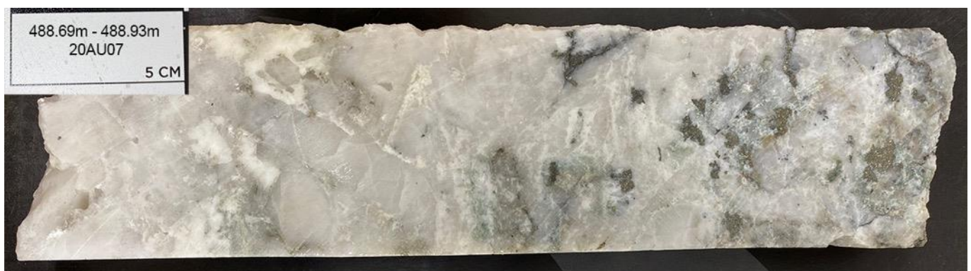
Figure 4 Hole #7 (20AU07) 488.69m - 488.93m quartz vein with fuchsite, arsenopyrite, pyrite and pyrrhotite
