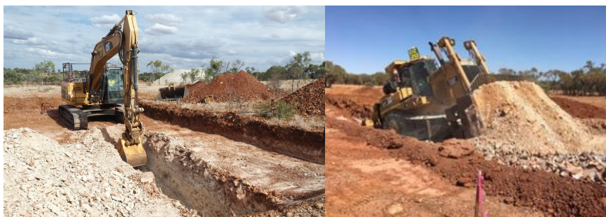
FIGURE: Ardmore mining trials; Excavator “free-digging” shallow phosphate rock (left), and dozer stripping shale overburden without the need for ripping (right).
