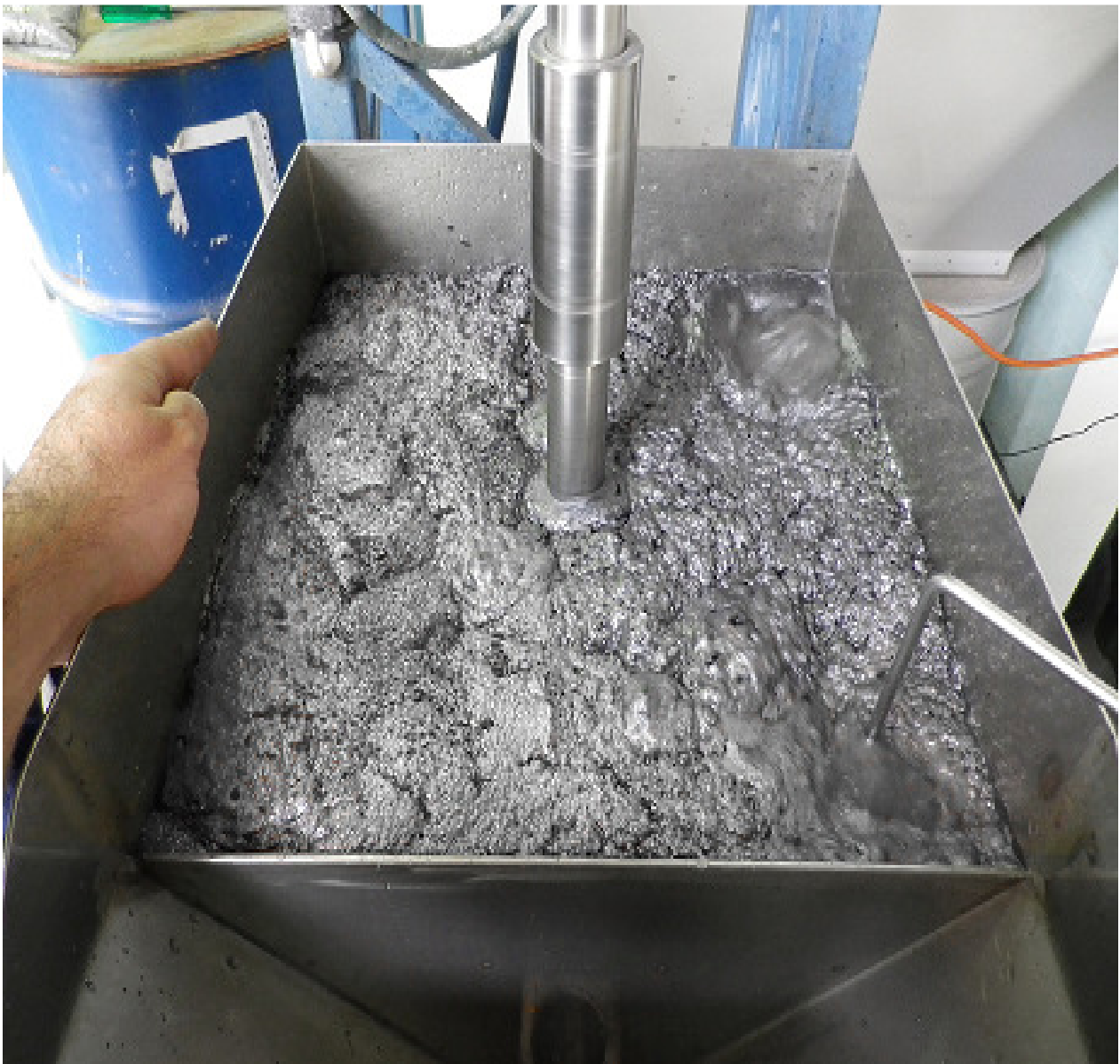
Figure 2: Larger Scale (60 L) Bulk Flotation Test
