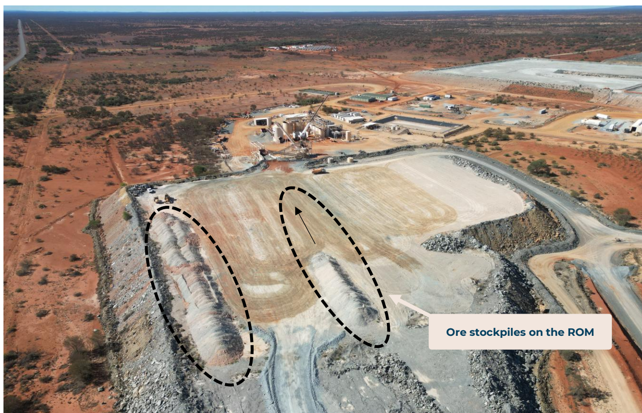
Figure 4: Ore stocks being built up on the ROM in preparation for process plant commissioning in June 2025.
