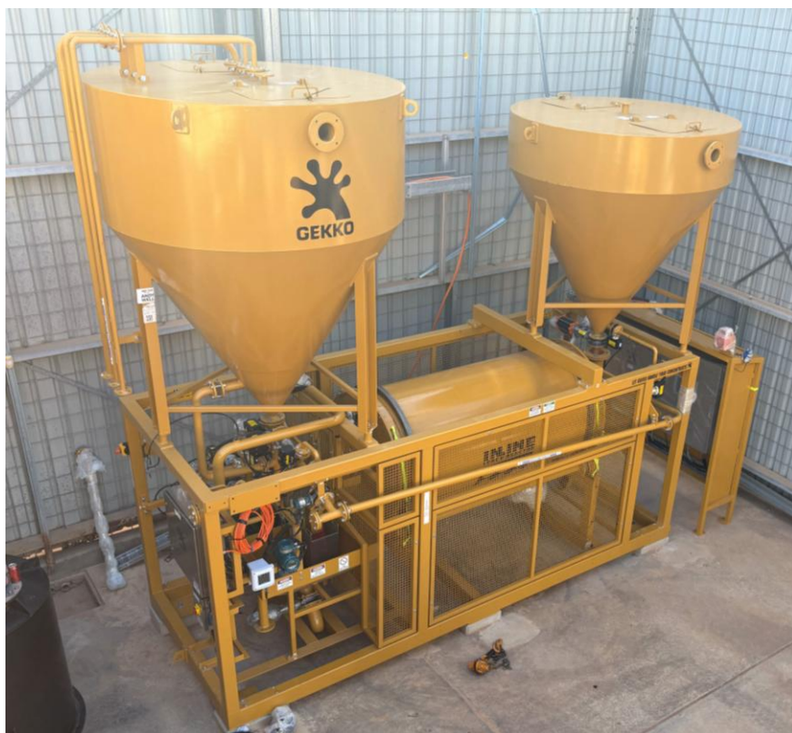
Figure 5: Installation of the InLine Leach Reactor (ILR), part of the gravity gold circuit, in the gold room, April 2025.
