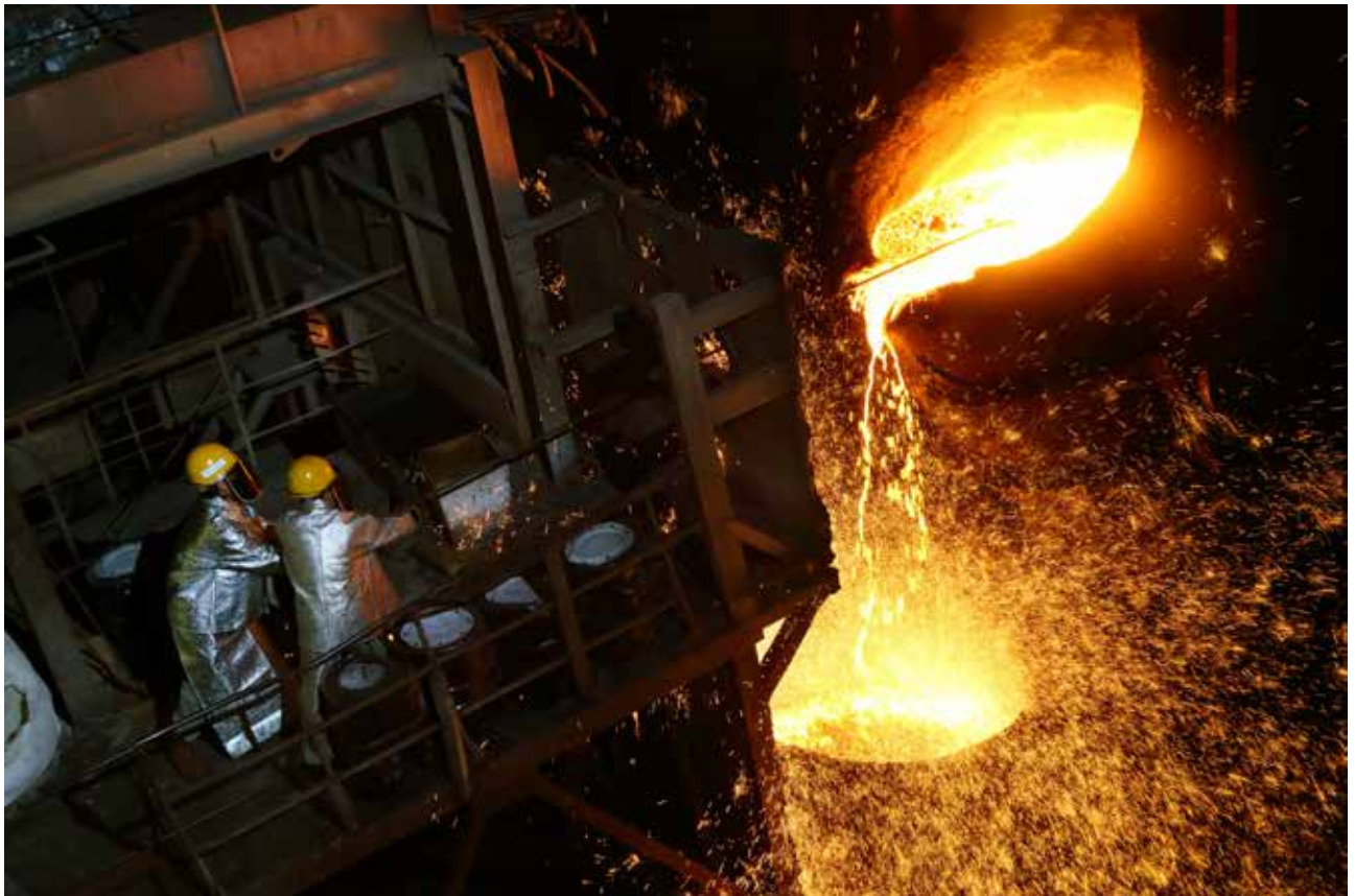
Proses produksi feronikel di pabrik feronikel di UBP Nikel Sulawesi Tenggara. The ferronickel production process in the ferronickel plant in Southeast Sulawesi Nickel Mining Business Unit
