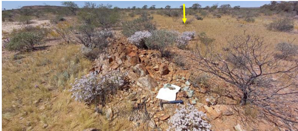
Figure 2. VMS base-metal target; malachite, azurite and chalcocite bearing exhalative barite lens. Arrow pointing to gossan block within trench. (Sample# ZEU016).
