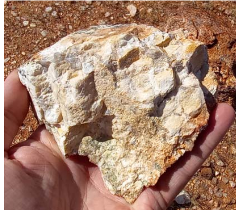
Figure 8. Albite-Quartz pegmatite from location of Figure 6. Sample location as sample # ZEU007.
