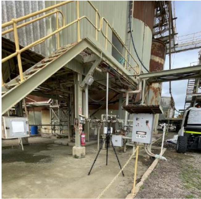
3D Laser Scanning Setup
