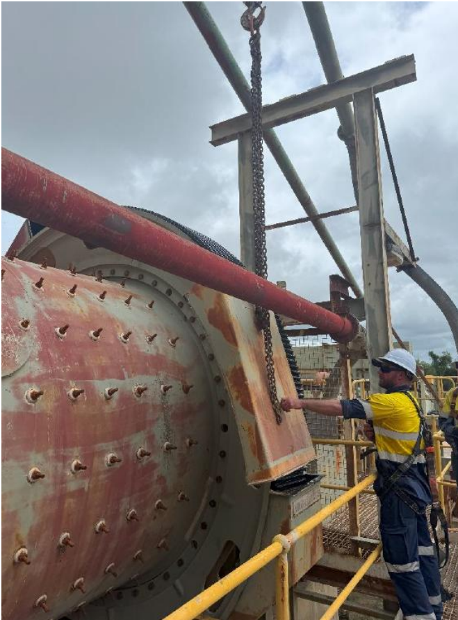
Removing of guarding for girth measurement
