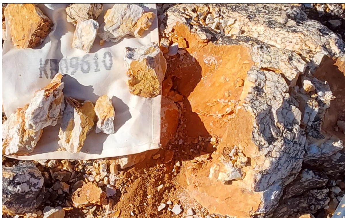
Photo 1 – Quartz vein outcrop rock chip resample returning 39.4g/t gold (KB09610), originally returning 22.5g/t gold rock chip assay (KB09374). Comprised of milky white, slightly bucky and brecciated vein quartz, with stockwork iron in fractures throughout and some limonite. Sample bag is 30 cm wide for scale.
