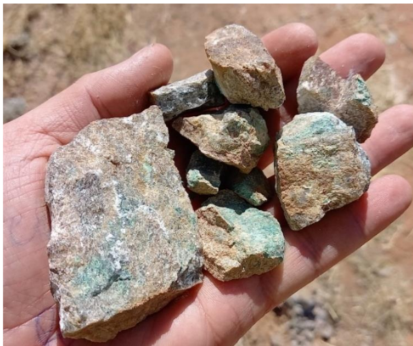
Figure 5. Detail of mineralised subcrop. (Sample# ZEU046 = 1.70% Cu, 01.51% Pb).
