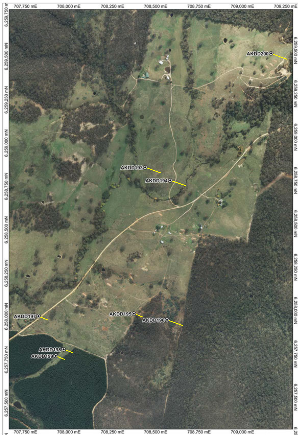
Figure 2 – Drillhole collar locations and planned hole traces shown on an aerial photo of Kempfield (plan view)
