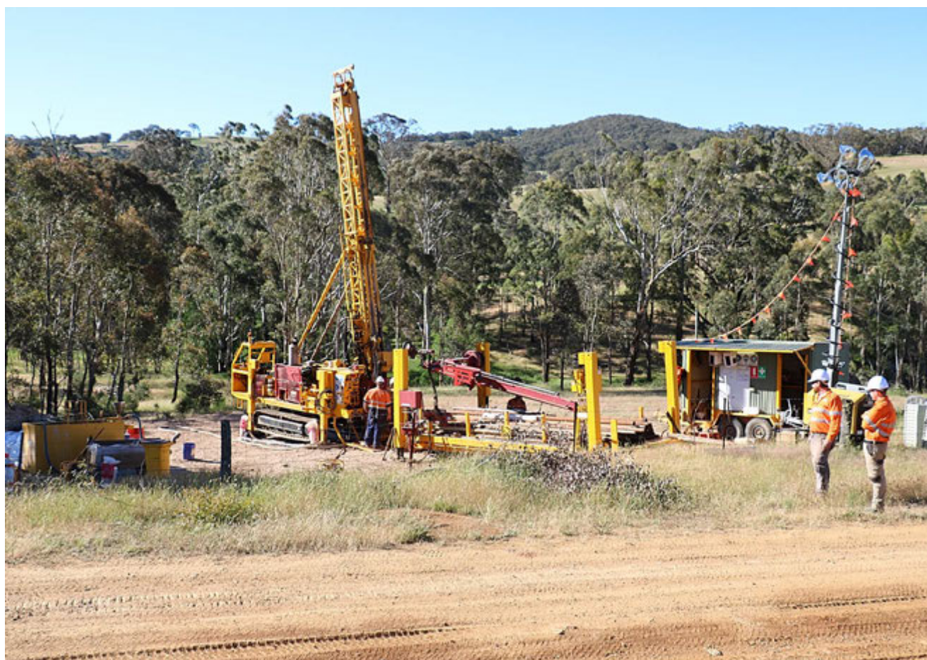
Figure 1 – Drill camp with diamond drilling in progress for the first hole of the programme, AKDD197.
