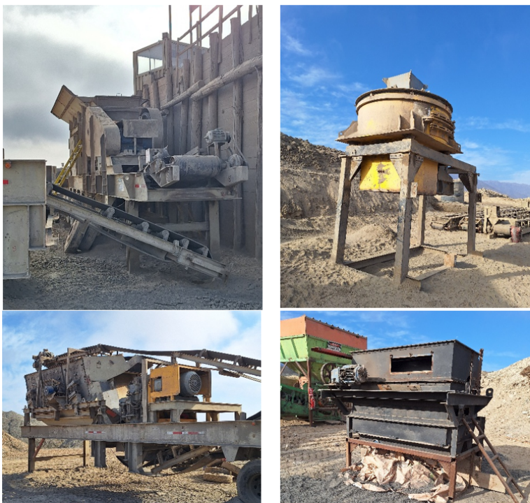
Images 2e-2h: The 3-stage crushing process and Magnetic drum used to produce bulk sample
