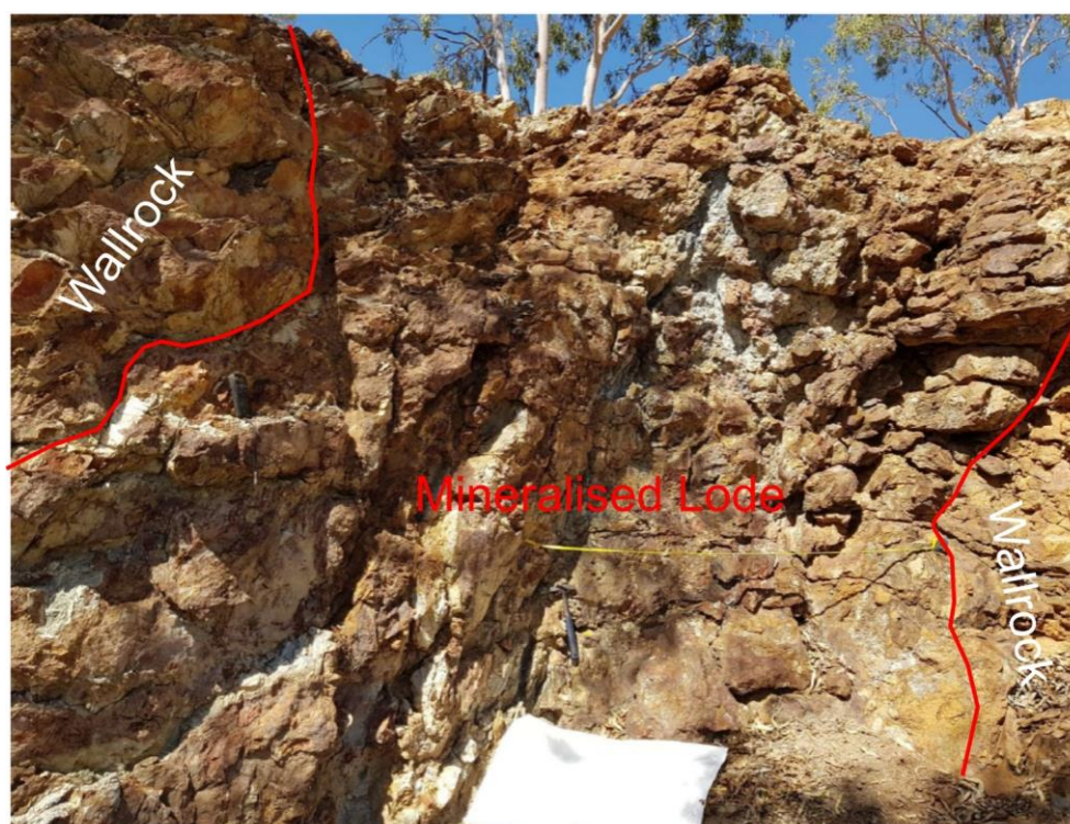
Figure 2: Gold mineralised lode in Lucky Break pit wall, face sample by QXR in late 2020, the 2.6m wide lode showed a length weighted average gold grade of 4.70 g/t Au (from 1.4m at 6.01 g/t Au and 1.2m at 3.17 g/t Au).
