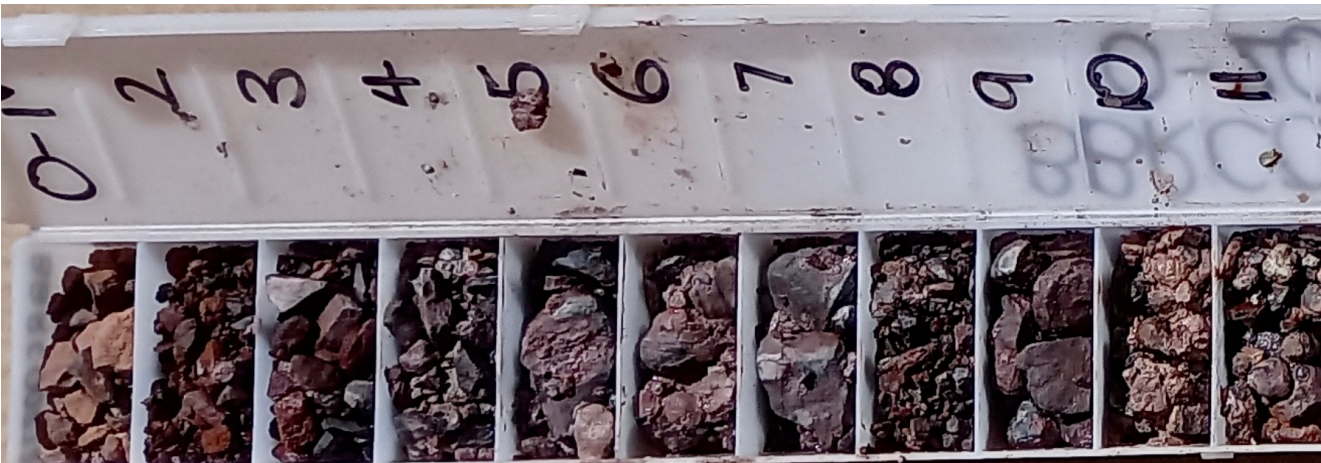
Figure 2. Lateritic manganese mineralisation intercepted in exploration drilling at the Butcherbird Project
