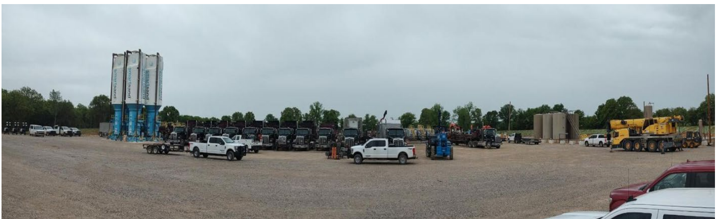
Figure 1: Completion crews and equipment mobilised on site at the Bruins Well. Infrastructure includes high-pressure pumps, sand silos, fluid storage units, and service vehicles ahead of 24-hour hydraulic fracturing operations.
