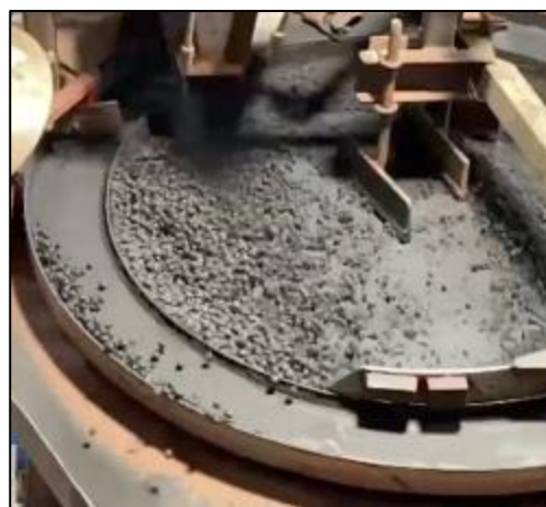
Picture 1. Green Ball manufacture in pelletising disc
