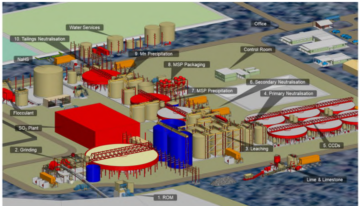
Figure 8 - 3D isometric of the Mt Thirsty processing plant showing generalised process flow (numbered labels)
