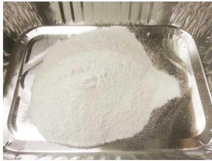
Figure 2. Sample of unwashed aluminum oxide produced during the Test Work
