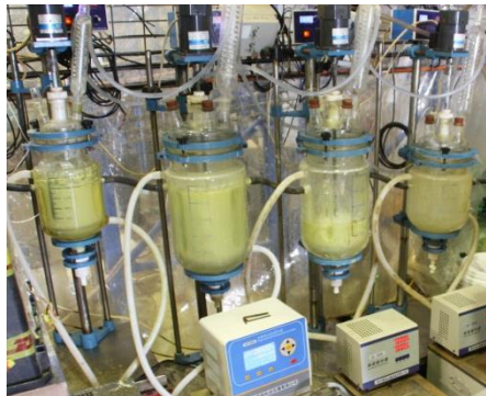
Figure 1. Leaching phase of AMMG's process conducted on a continuous basis
