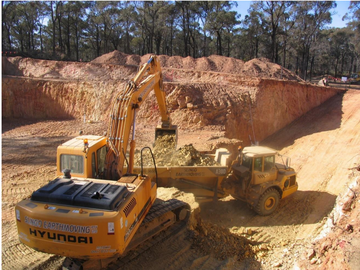
Figure 4: Excavating Bulk Sample Pit at Harvest Home
