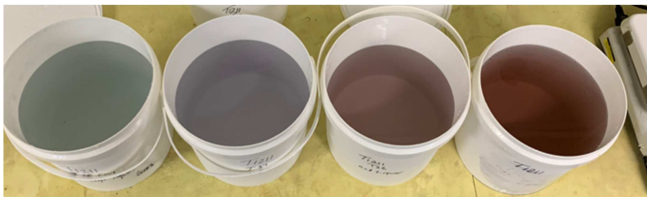
Figure 6: Progressive extraction of copper from Pregnant Leach Solution (PLS) (PLS in bucket second from left showed maximum copper extraction with minimum cobalt loss)
