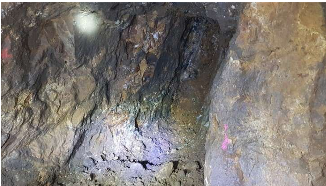
Figure 2 - the face of the Mystery Drive showing the extension of the vein before sidewall waste is removed
