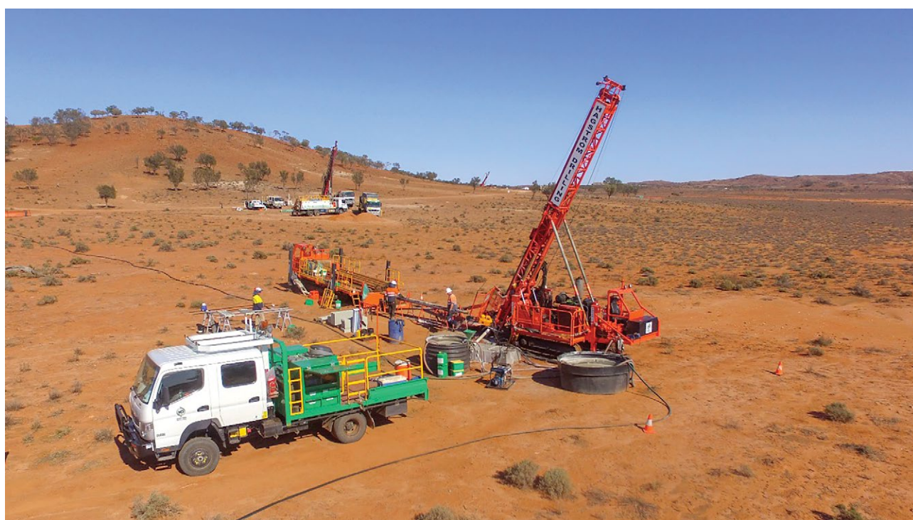
Figure 1. Diamond and Reverse Circulation drilling operations at Pyrite Hill.
