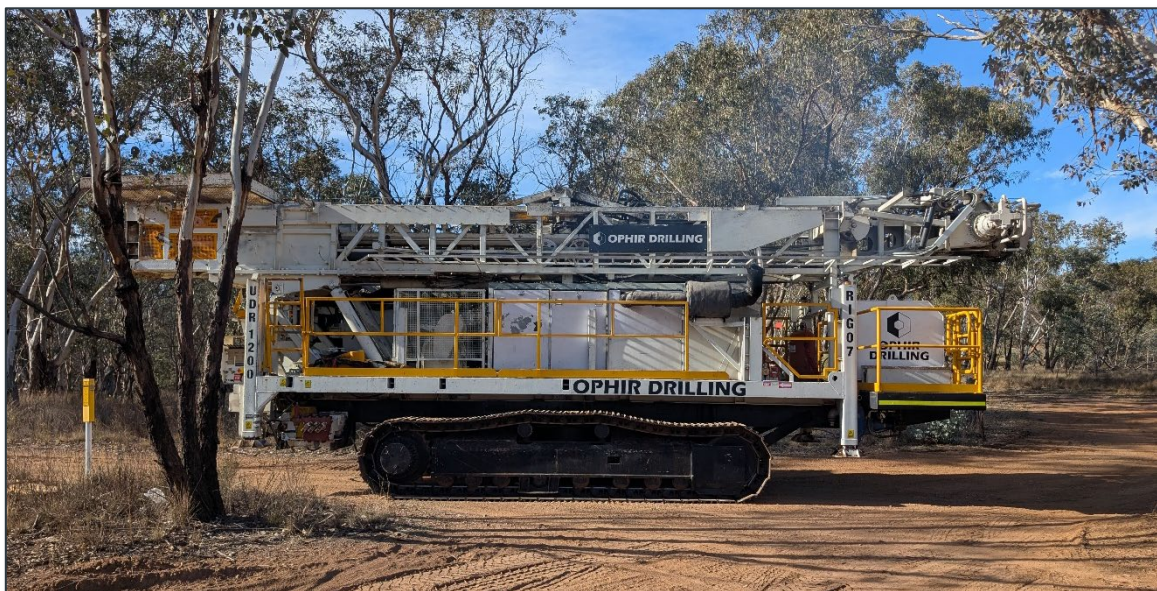
Figure 1: Diamond drill rig mobilising to the Breccia West Prospect
