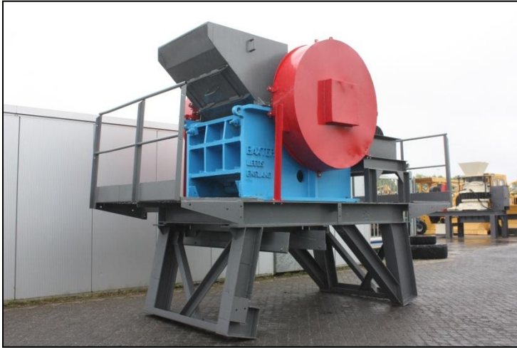
Typical primary jaw crusher
