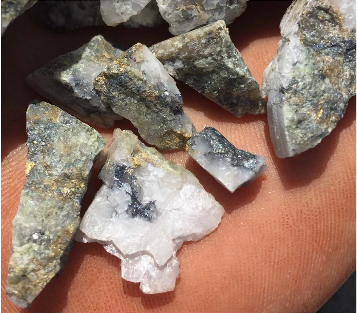
Figure 2 Example of visible gold at 586m depth in MSDD156
