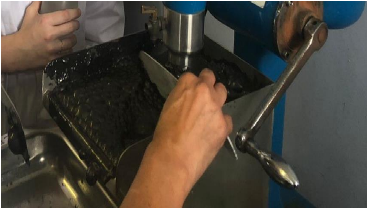
Figure 2: Carbon flotation indicates high flotation kinetics
