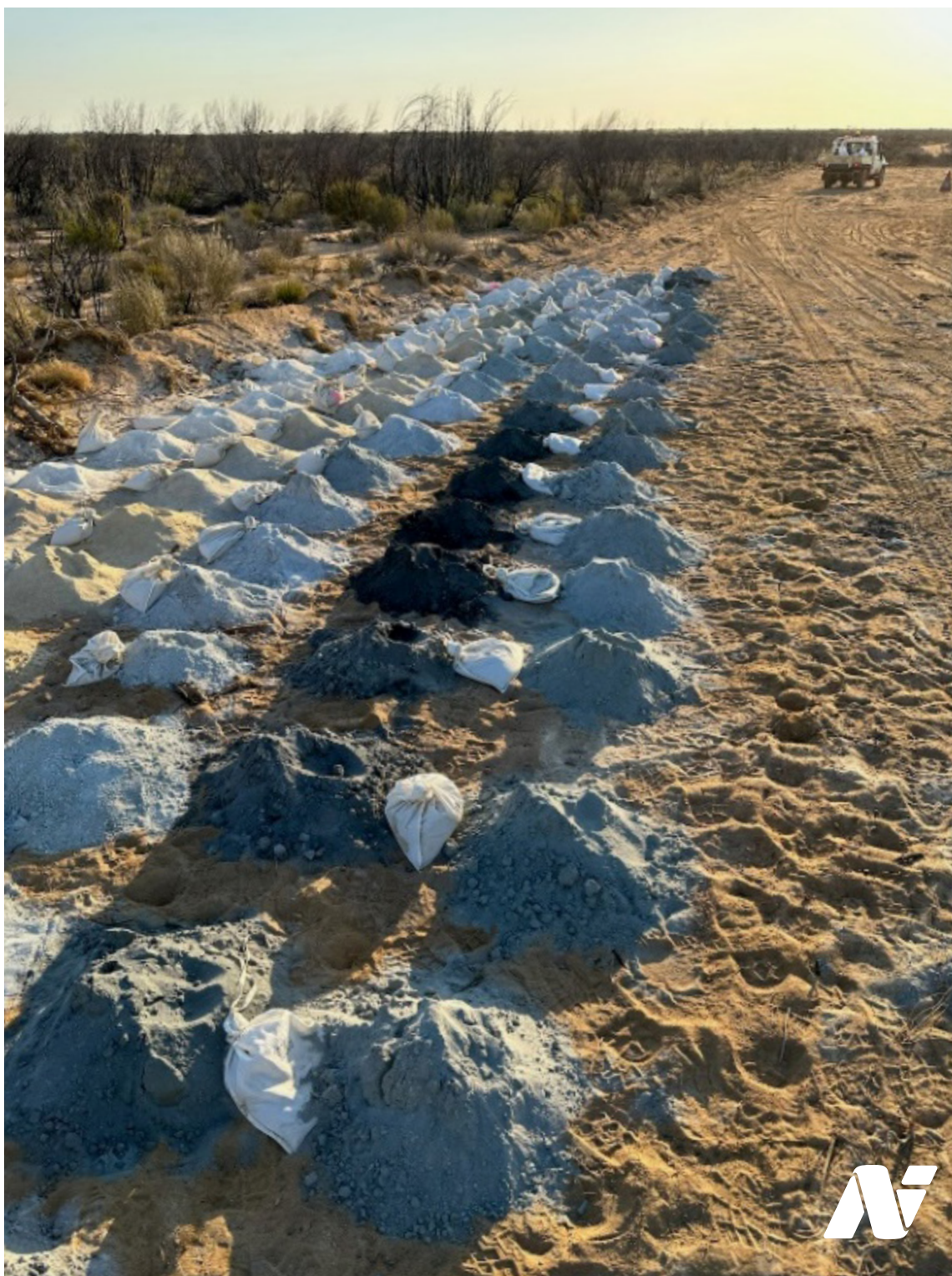
Figure 3 – 23NRRC100 R/C Drill Piles, black material represents massive sulphide intersections.
