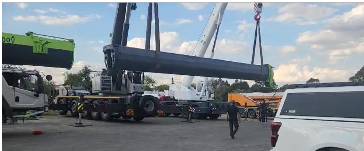
Figure 6: 200-tonne crane disassembly in Johannesburg, South Africa. for transport to site
