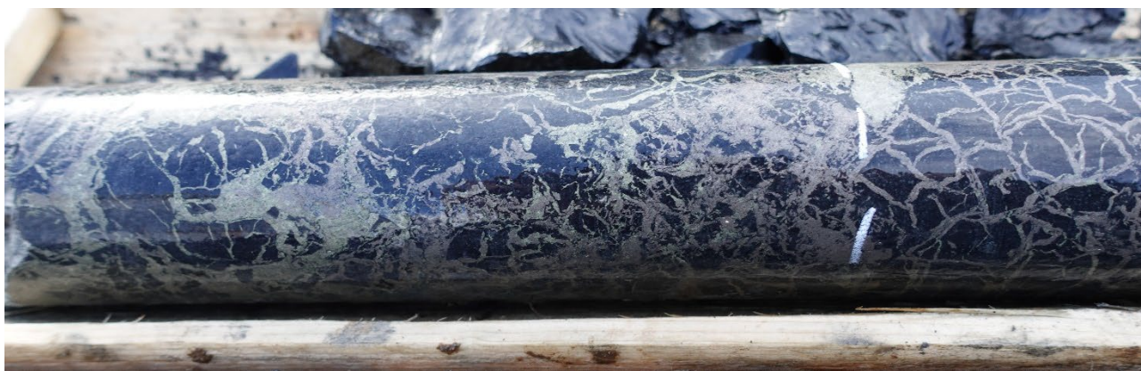
Figure 6: YH24-126 - 170.20-170.70m, 3.16% CuEq - 3.09% Cu, 0.11% Zn, 12.1g/t Ag
