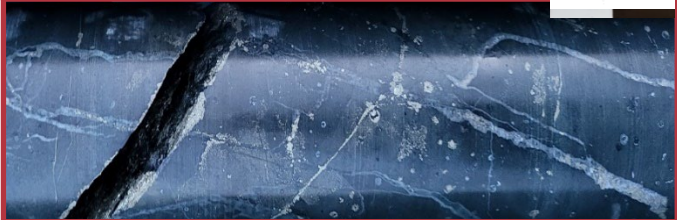
SPD003 419.8m, pyrite stringer stockwork/multiple vein sets associated with silica alteration, 1.42g/t Au (Epithermal)
