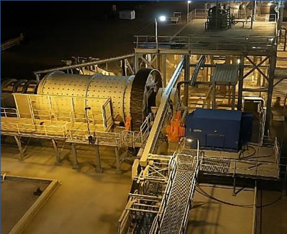
Figure: Existing 1800kW Ball Mill
