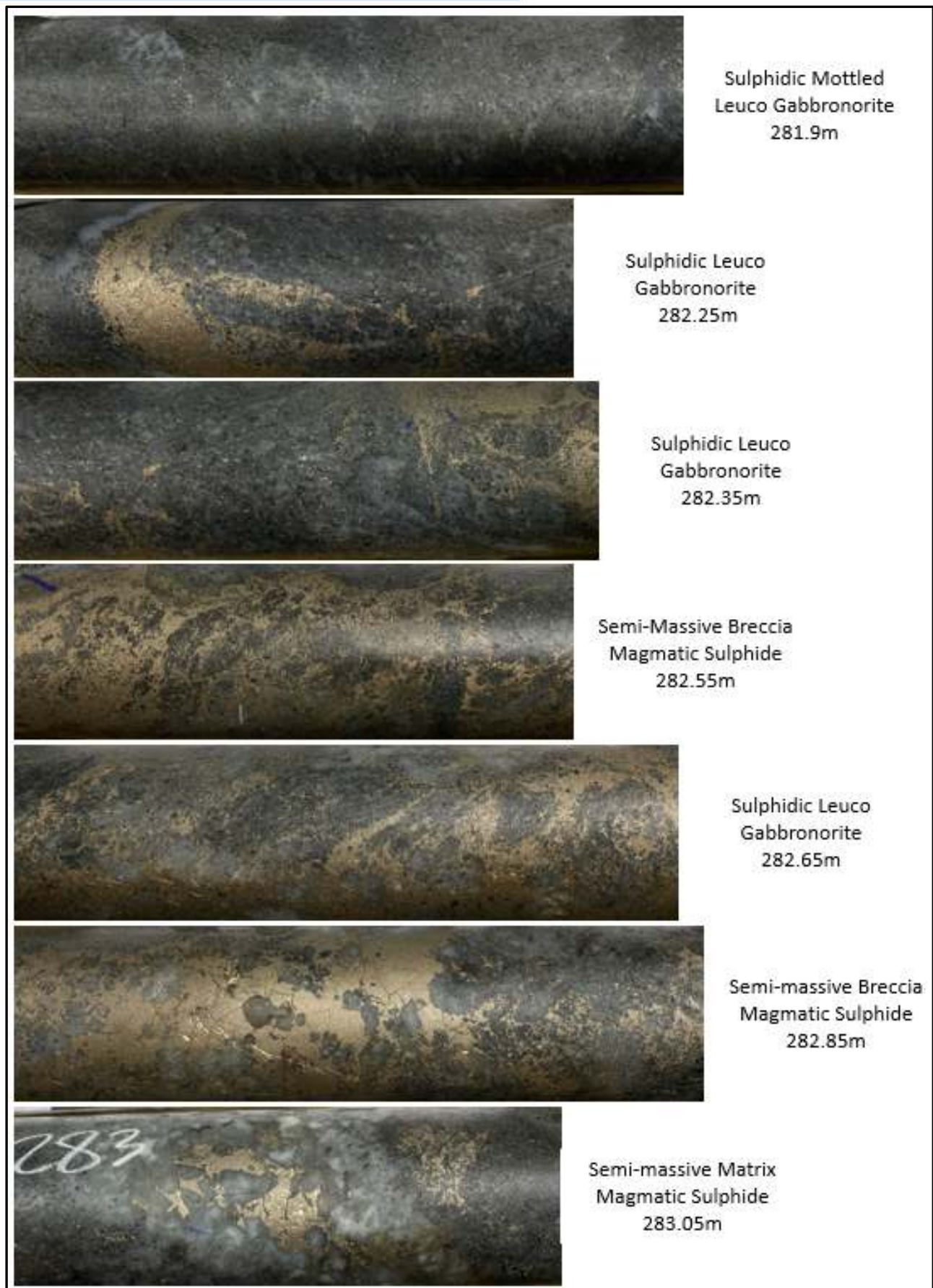
Figure 2 – Core photos of sulphide zone at about 282m downhole
