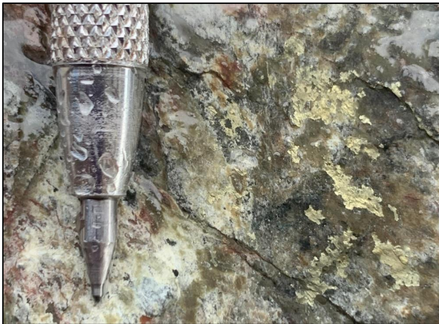
Figure 4. Trace chalcopyrite (copper mineral) on joint surface at 427.3m.
