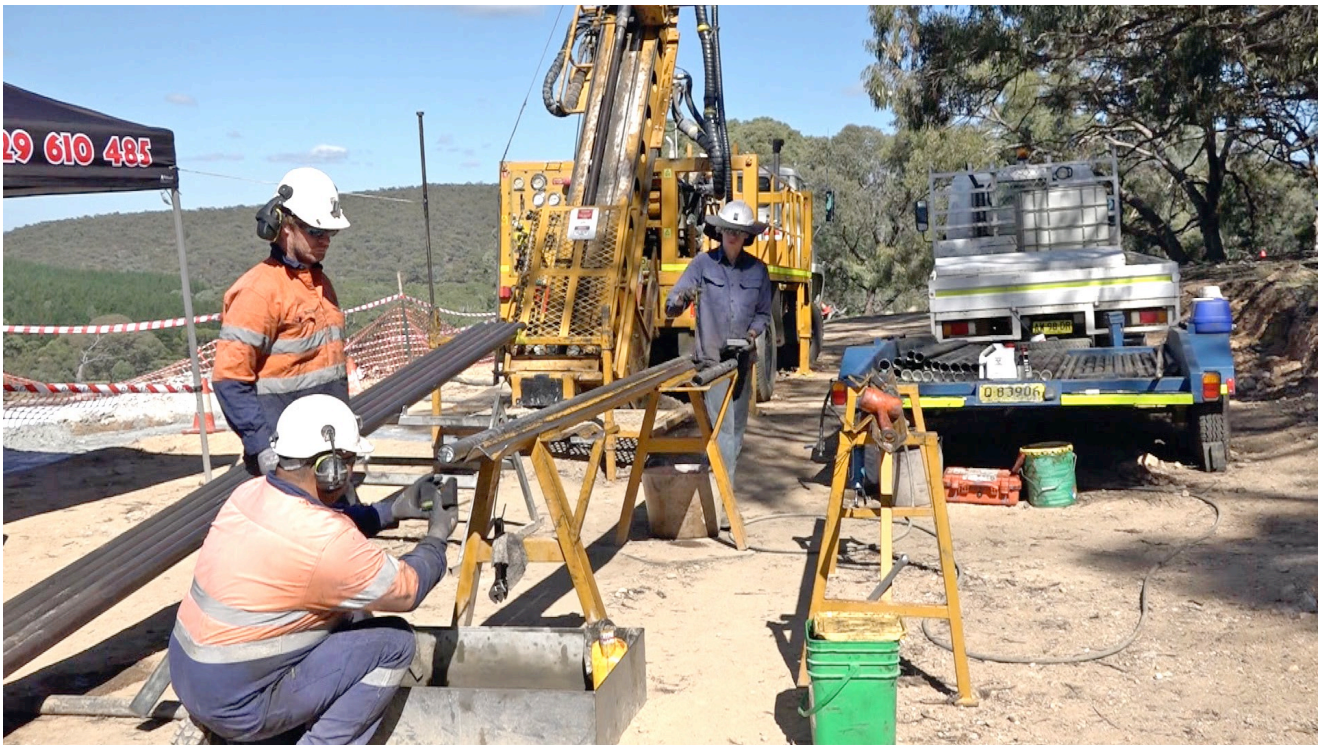
Figure 2 - Electronic orientation information is marked on a section of diamond core for Hole #1
