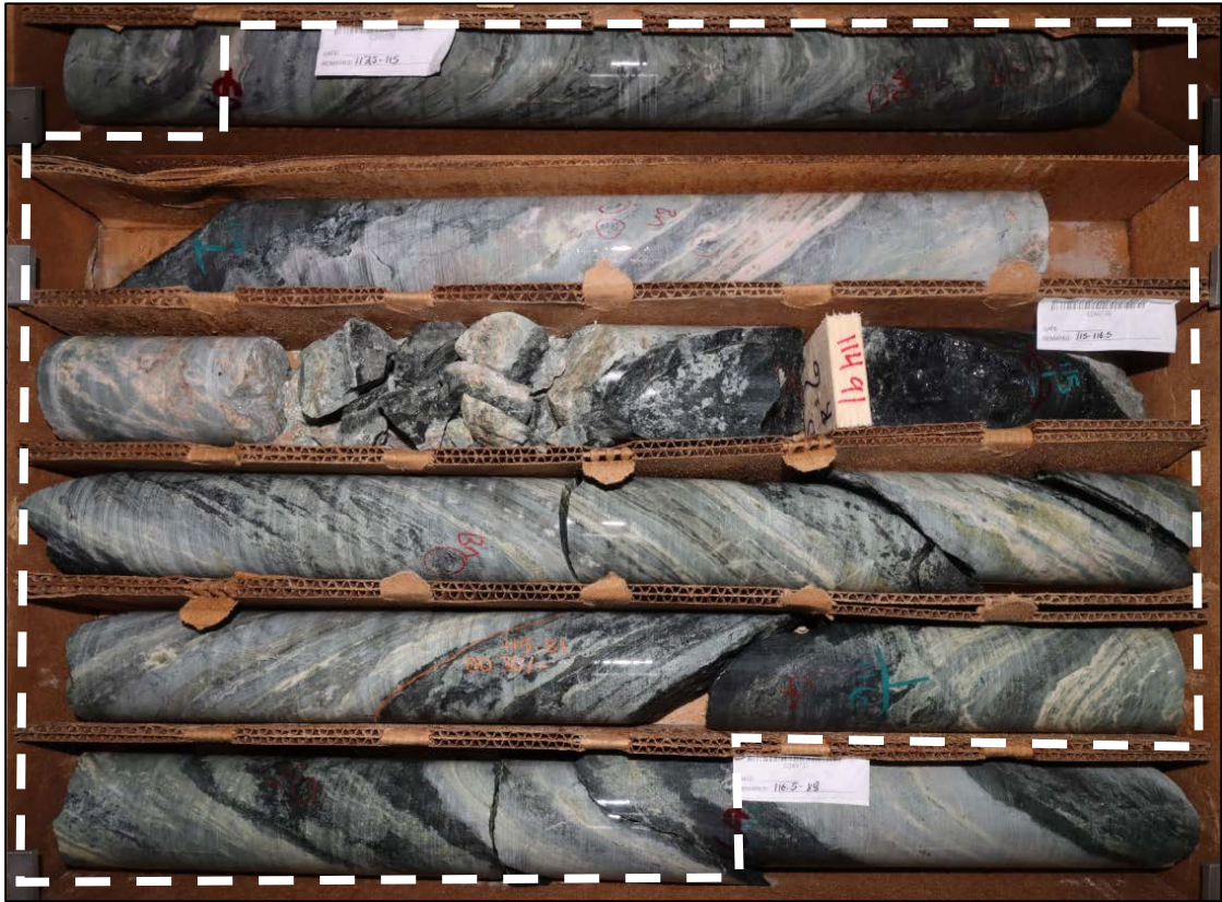
Figure 5 – Example of moderately to weakly mineralised zone in WT-21-24 within banded sediments. Outlined interval averages 3.0m at 0.44% Cu, 3.10g/t Ag, 0.07g/t Au (113.5 to 116.5m)
