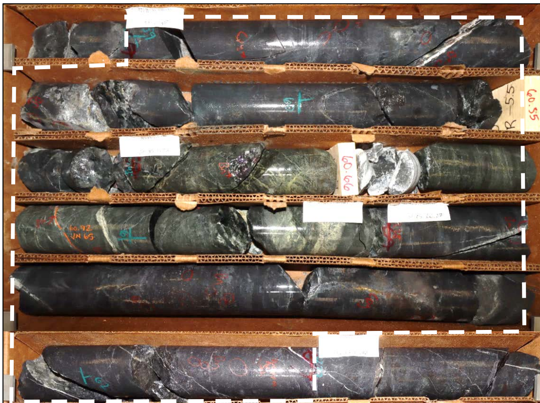
Figure 4 – Example of strongly mineralised zone in WT-21-24 with magnetite-rich skarn. Outlined interval averages 3.3m at 4.16% Cu, 43.65g/t Ag and 0.70g/t Au (59 to 62.3m)
