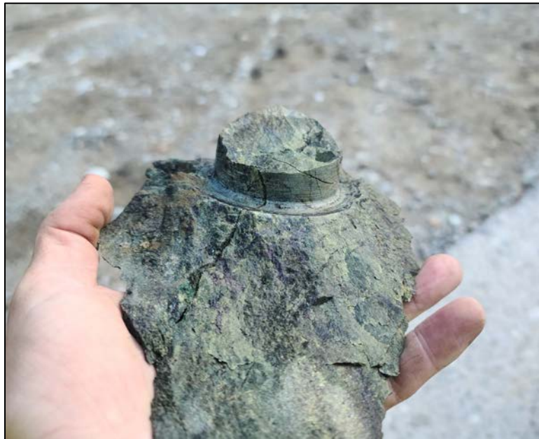
Figure 3- WT-21-24 pierce point through existing underground development. The drill hole encountered strongly altered and mineralised material just before piercing through the historical mine. Note the rounded mark from the diamond core drill bit at the top of the specimen.
