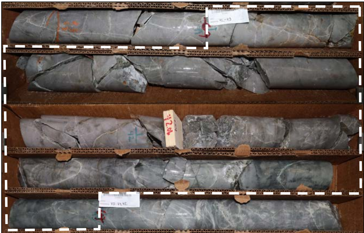
Figure 6 – Example of unmineralised zone in WT-21-24. Outlined interval averages 2.0m at 0.01% Cu and 0.19g/t Ag (41 to 43 m)
