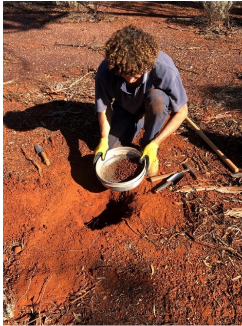
Figure 2: Soil samples sieved to -2mm passing on site.
