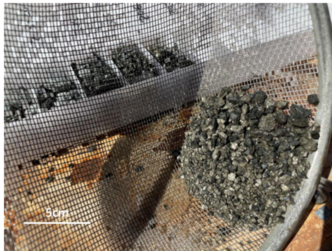
Massive sulphide chips in MIRC013 from 207-208m (pXRF 0.7% Cu and 0.2% Ni)
