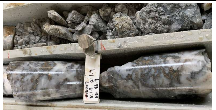
Figure 8 – HUD007 – 87m – Quartz-sphalerite vein
