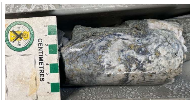
Figure 4 – HUD005 – 50m – Quartz-galena-sphalerite vein
