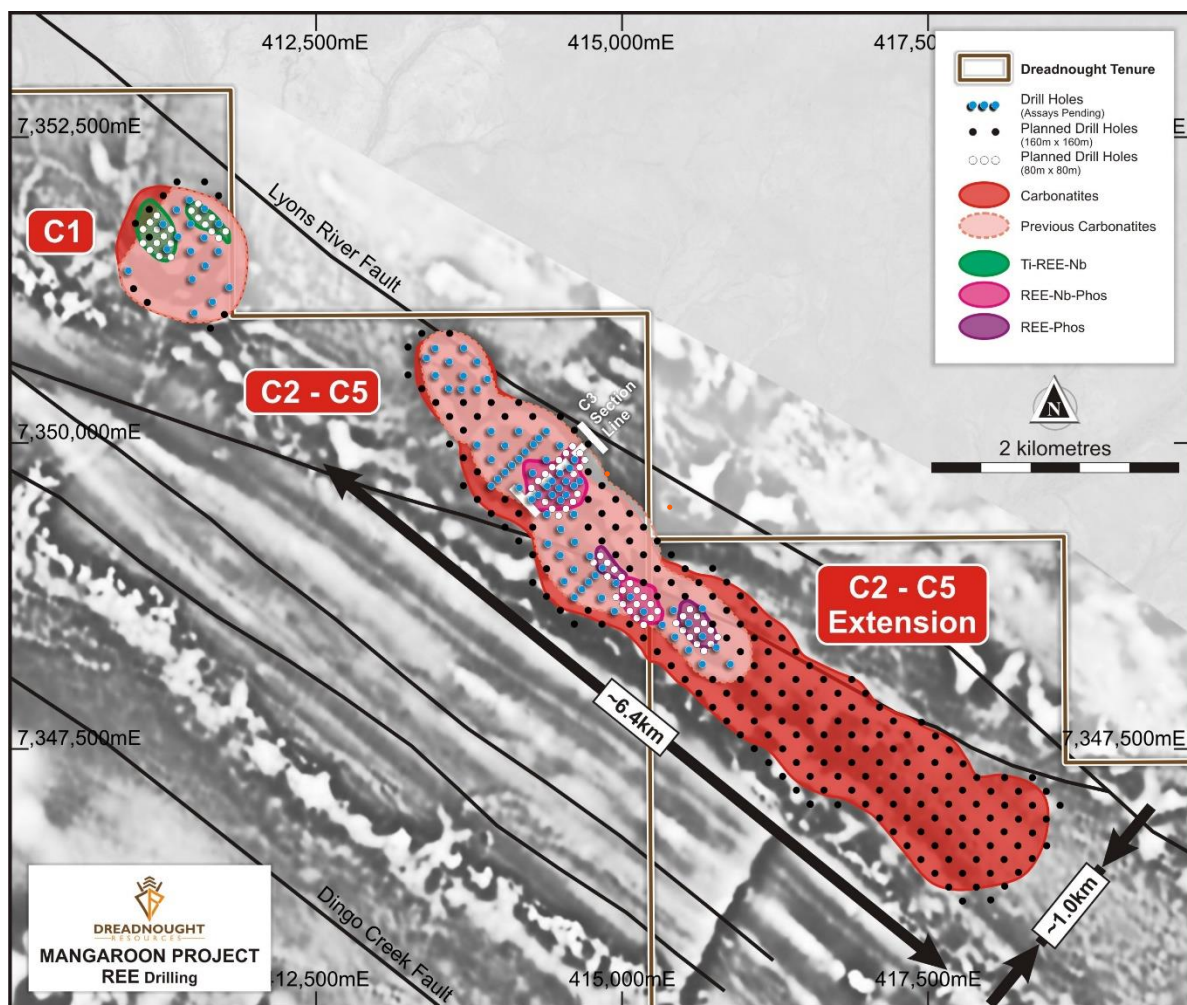
Figure 2: Plan view of the C1-C5 carbonatite intrusive complex highlighting the zones of REE-Nb-Ti-P identified to date. Also shown are planned 80m x 80m spaced angled infill holes (white) and 160m x 160m vertical holes over the extended carbonatite zone (black). C6 and C7 are off image – both remain untested.
