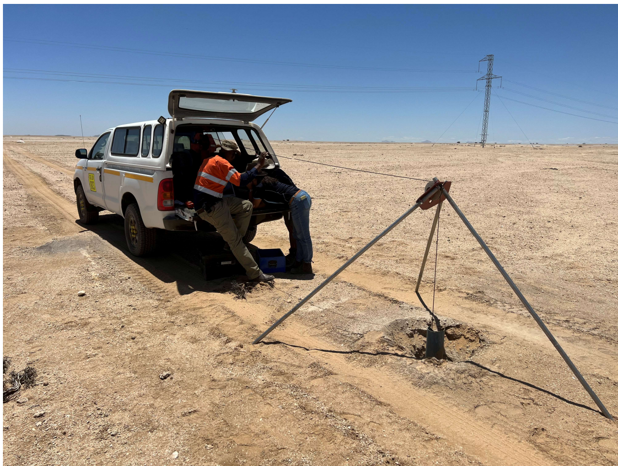
Figure 4 Downhole Gamma Probing at Koppies 3
