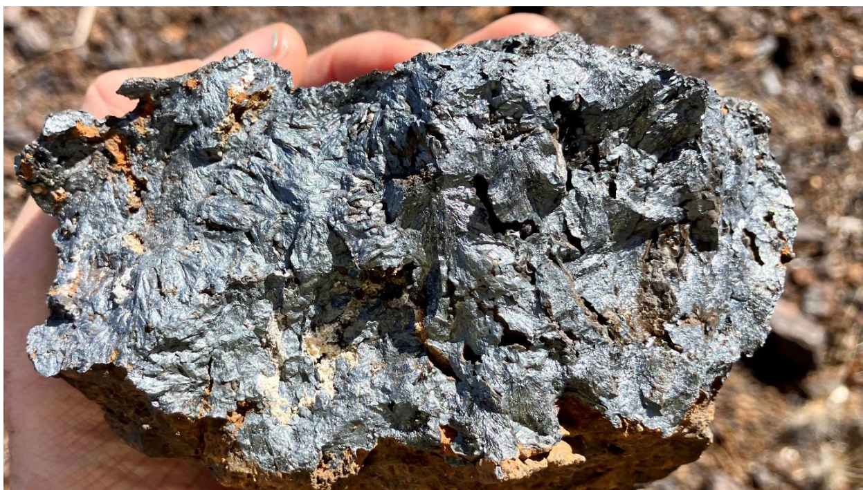
Figure 7. Manganite sample showing pyrolusite needles (Sample#ZEU110).
