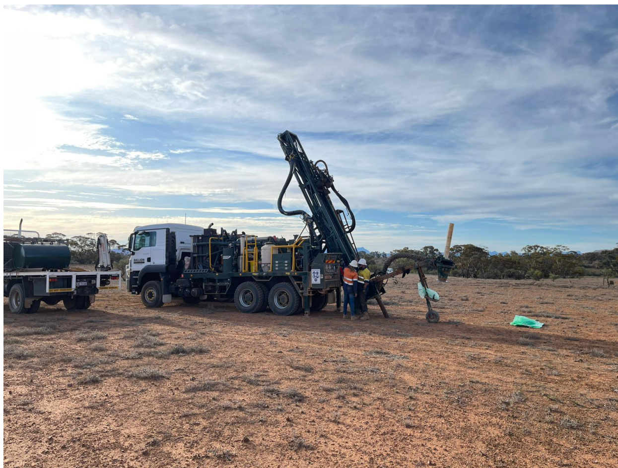
Photo. RAB drilling underway at Mt Craig
