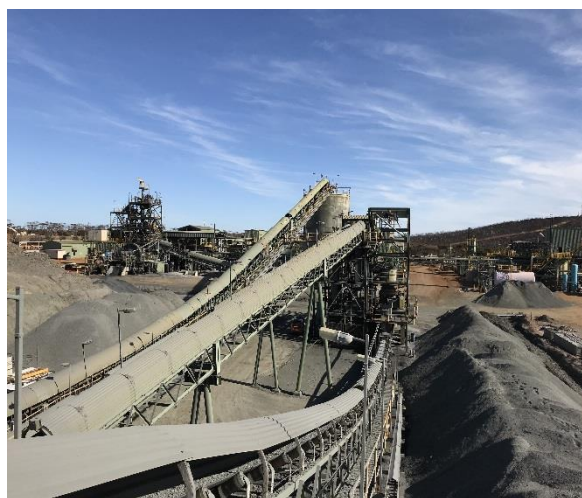
Crushing circuit conveyor to Fine Ore Bin (FOB)
