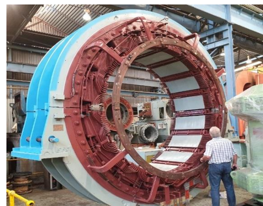
Fully Reconditioned Stator at Marthinusen & Coutts
