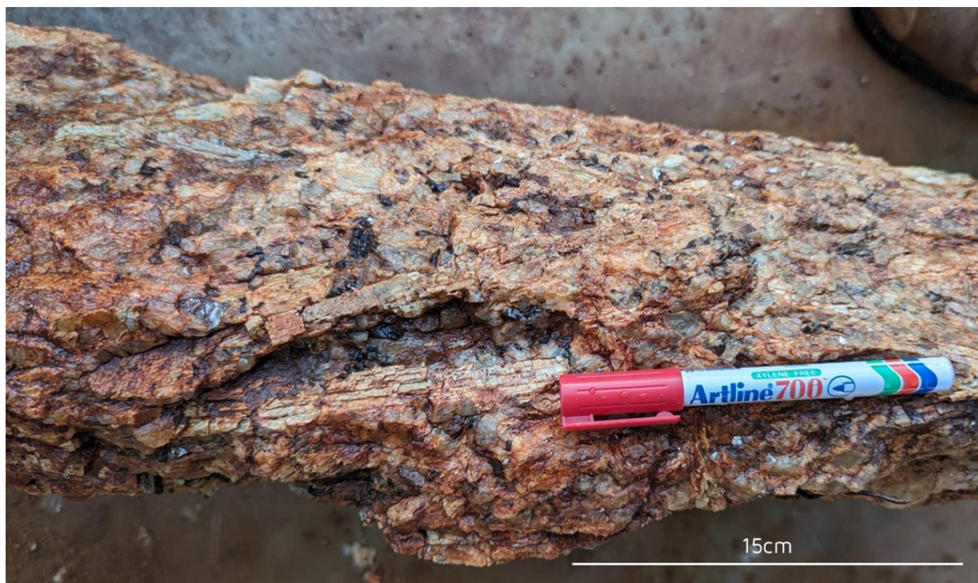
Figure 3 – Pegmatite subcrop sample with coarse spodumene crystals from the Bird Rock Prospect.
