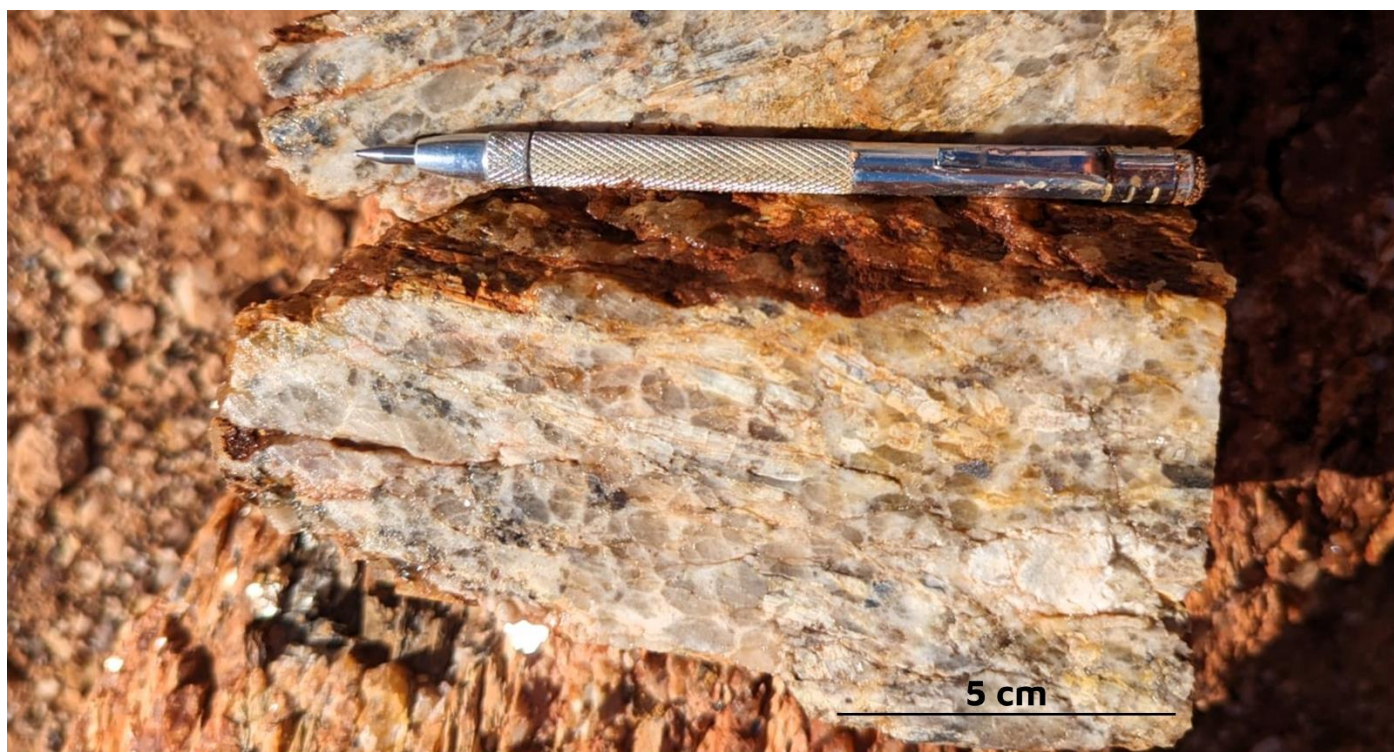
Figure 4 – Coarse spodumene crystals from the Bird Rock Prospect grading 3.54 % Li 2 O (SMX00887).
