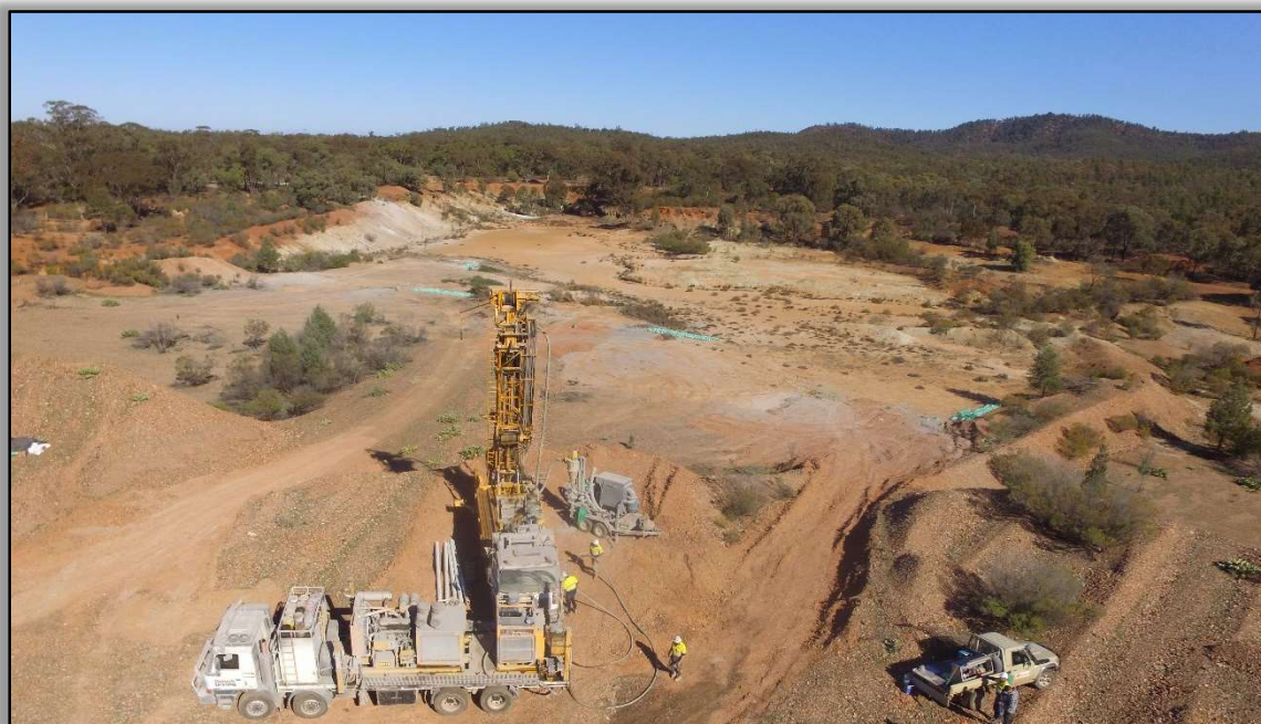
Figure 1: Oblique aerial view of RC drilling rig, showing extensive historic Tallebung open cut workings in background
